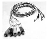
The fused potential leads provides the technician protection when measuring a higher system voltage (600 vac/2 amp fuse). Set of 4 fused leads, 6 ft. 6 in. (2m)
